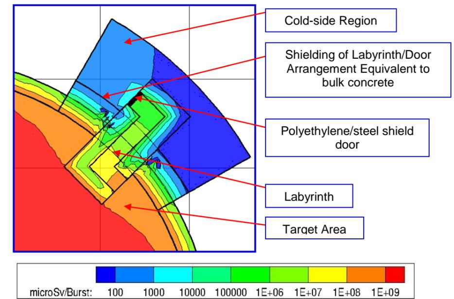
The assessment demonstrated that there is significant scope for providing high levels of shielding for personnel access doors through the use of labyrinths in combination with shield doors based on a compound polyethylene (neutron) and steel (gamma) shielding construction.
